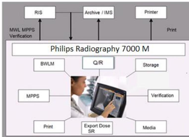
**Figure 1: Radiography 7000 M in a DICOM network**
