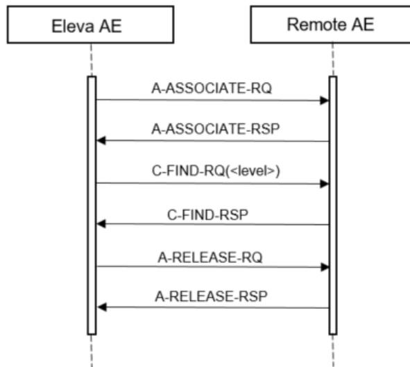
Figure 12: Data Flow Diagram – FIND as SCU
