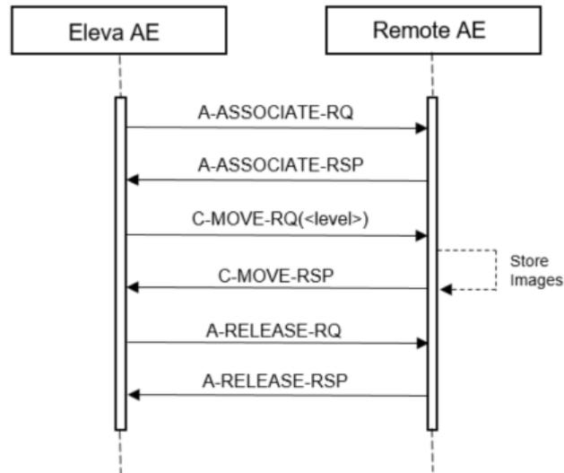
Figure 13: Data Flow Diagram – MOVE as SCU
