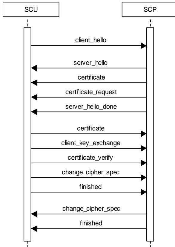
Figure 17: Message flow of TLS handshake
